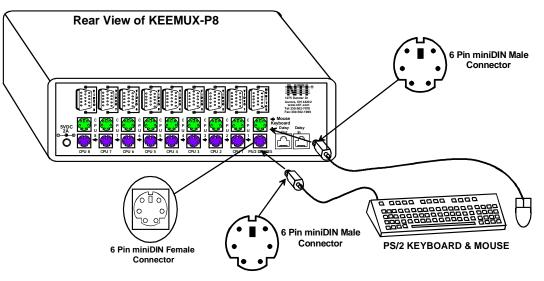
Figure 3- Connect the user keyboard and mouse
